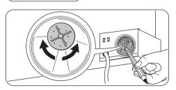
Check carefully whether the pump impeller rotates (it rotates jerkily). If it doesn't rotate, please contact your Service Centre.
